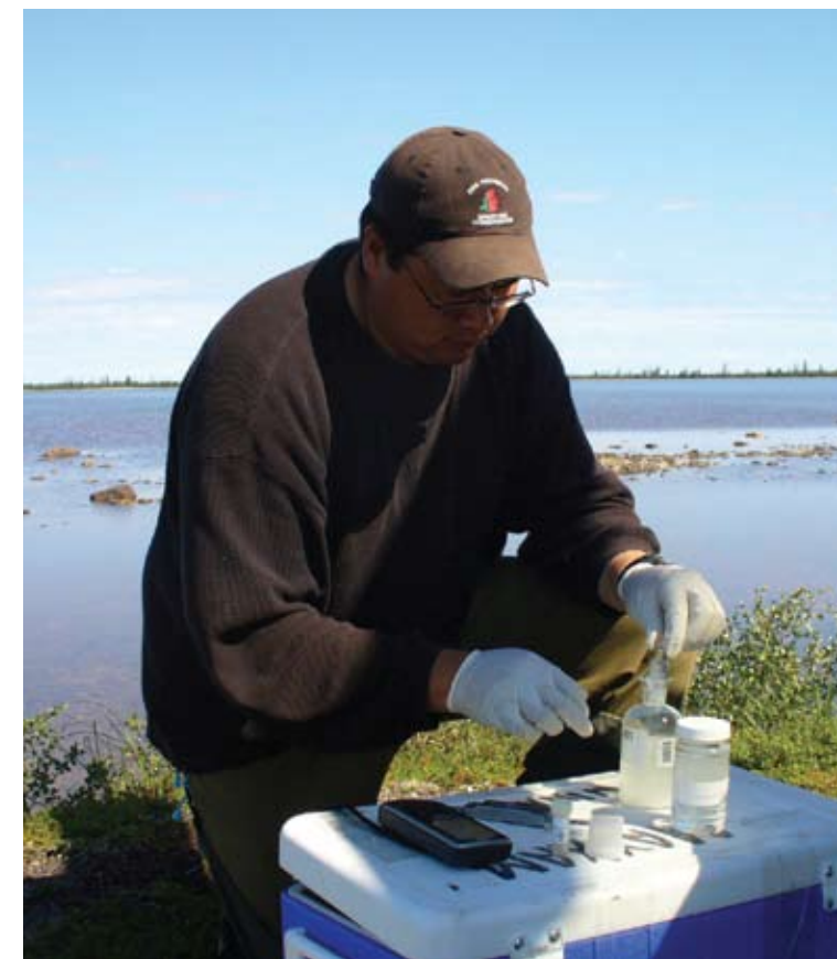
Rodney Redhead taking an in-situ water measurement at Mary Lake using the YSI 556 multimeter. Photo: Mike Taylor
