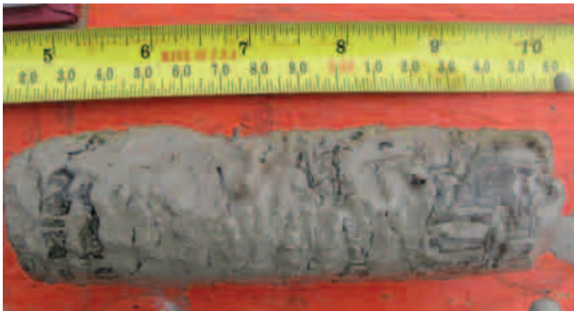
Drill core showing ice lenses in mineral soil found below peat in a peat plateau. Scale in centimetres and inches. Credit: Wendy Sladen.
