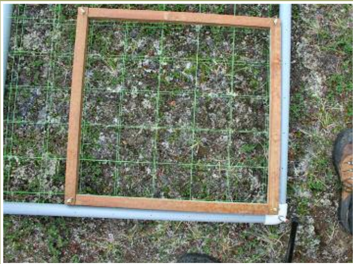
Three nested vegetation sampling methods: 1) expert ITEX point frame (grey frame with green threads) for detailed but time-consuming sampling; 2) non-specialist percent (%) cover in the field using a small brown frame without threads for faster, less detailed assessment; and 3) taking photos of the frame using a tripod and camera: very quick but captures only the top layer of vegetation. Credit: Parks Canada, Chantal Ouimet
