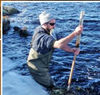
Dr. Frédéric Bouchard collecting surface sediments with a simple device (hand-held coring tube), September 2012 Credit: Lauren MacDonald
